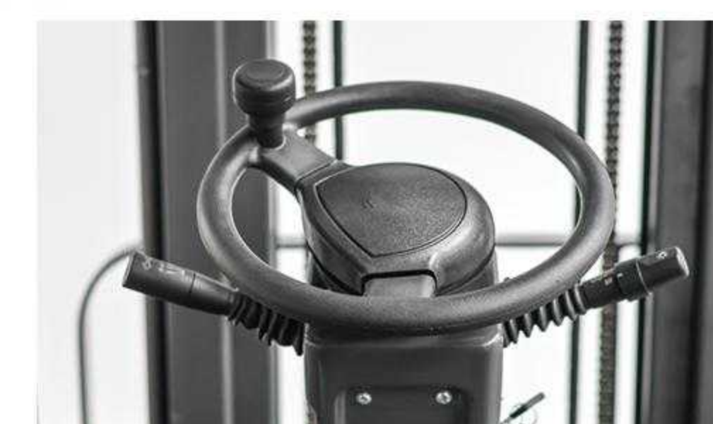
Hydraulic steering operation
