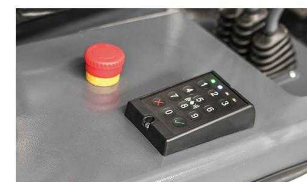
Emergency switch + Pin-code lock
